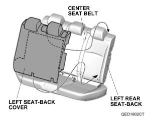
5. Secure the fasteners to the left rear seat-back.
