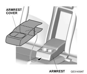
9. Raise the armrest. Pull out the armrest cover between the armrest and left rear seat-back and secure the fasteners to each other as shown.
