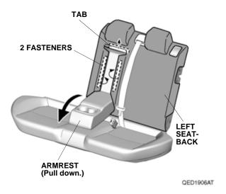
3. Pull up the armrest. Secure the fasteners to the left rear seat-back. Go to step 6.
