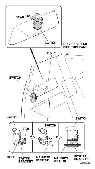
34. Align the tab on the switch bracket to the hole on the switch and secure the switch bracket to the switch with one narrow wire tie.
