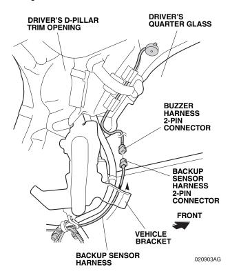
46. Plug the backup sensor harness 2-pin connector to the buzzer harness 2-pin connector.
