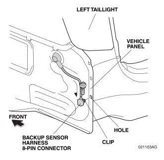
72. Secure the clip on the backup sensor harness to the hole on the vehicle panel as shown.
