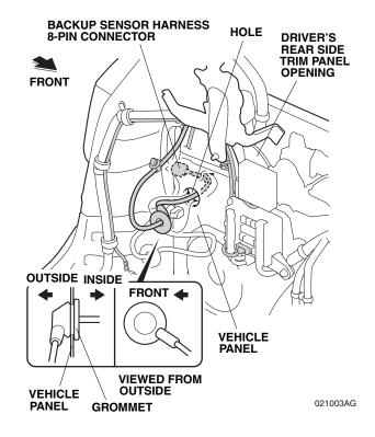
64. Route the backup sensor harness 8-pin connector, and secure the clip on the backup sensor harness 8-pin connector to the hole on the vehicle panel.
