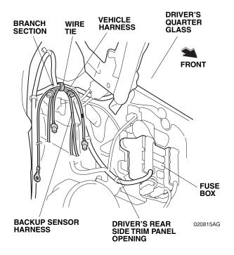
42. Route the backup sensor harness ground terminal along the vehicle harness.
