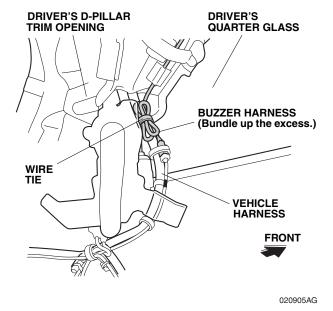
Route the backup sensor harness along the vehicle harness, and secure it to the vehicle harness with one wire tie as shown.
