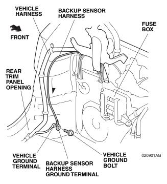
43. Remove one vehicle ground bolt and secure the backup sensor harness ground terminal to the vehicle ground terminal with the vehicle ground bolt just removed.
