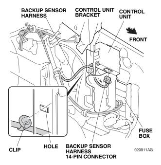
Secure the clip on the backup sensor harness to the hole on the control unit bracket as shown.
