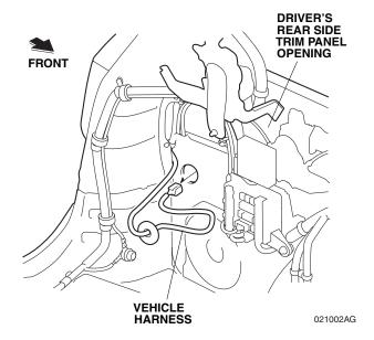
63. Route the backup sensor harness 8-pin connector through the hole, and secure the grommet on the backup sensor harness to the vehicle panel as shown.
