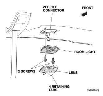
8. Remove the room light and unplug the vehicle connector.
