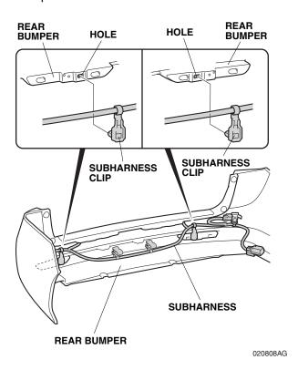
27. Secure two subharness clips to two ribs on the rear bumper as shown.
