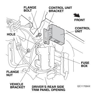
58. Route the backup sensor harness 14-pin connector, and plug it to the control unit.
