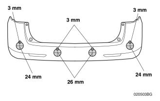
17. From outside of the rear bumper, while wearing eye protection, drill eight holes with a 3 mm drill bit. NOTE: Make sure to drill perpendicularly to the rear bumper.
