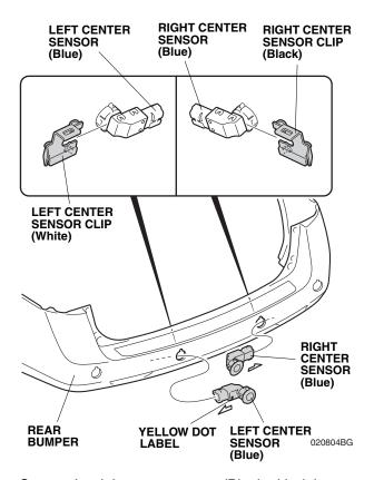
21. Secure the right center sensor (Blue) with right center sensor clip (Black) and the left center sensor (Blue) with left center sensor clip (White) as shown.
