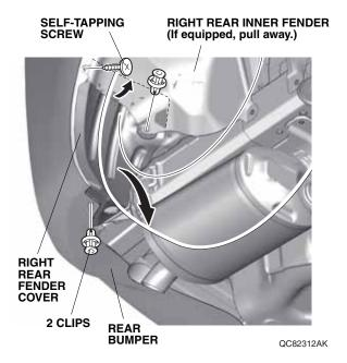
19. Locate the recessed mark. Using a pushpin, pierce the right rear fender cover at the recessed mark.
