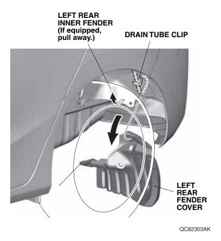
7. Locate the recessed mark. Using a pushpin, pierce the left rear fender cover at the recessed mark.
