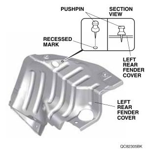
8. While wearing eye protection, drill the left rear fender cover at the pierced mark using a 3 mm drill bit first, then a 6 mm drill bit, 8 mm drill bit, and finish using a 10 mm drill bit.
