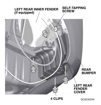
6. Remove the left rear fender cover, and drain tube clip.
