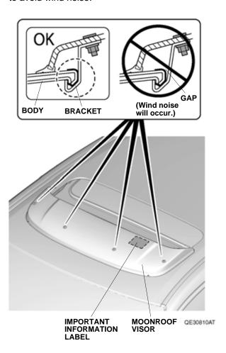
Position the moonroof visor with equal spacing in the front and on the sides. Check that the rubber molding is not twisted or rolled under the moonroof visor.
