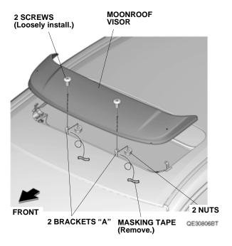
11. Loosely install the moonroof visor to left and right brackets "B" with two screws and two nuts. Remove the strips of masking tape from left and right brackets "B".
