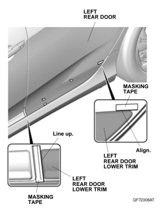
14. While applying light pressure against the left rear door lower trim, carefully remove the taped adhesive backings.
