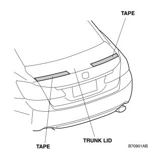
11. Place the template on the trunk, and align it with the left edge of the trunk lid. Tape the template to the trunk lid with masking tape.
