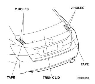
26. Enlarge the four holes made in the trunk lid in step 20 with a 7 mm hole cutter. Drill perpendicularly to the trunk lid.
