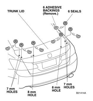
31. Remove the adhesive backings from the other end of the six seals.
