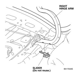
44. Remove and discard the two holders from the hinge bracket.
