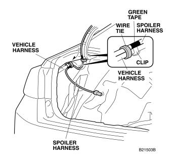
53. Secure the spoiler harness to the vehicle harness with five additional wire ties as shown.
