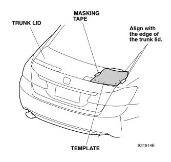
14. Using a felt-tip pen, mark the trunk lid through the hole in the template. Remove the template.
