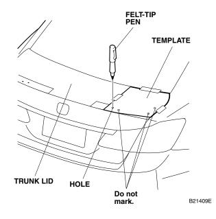
15. Using a center punch, punch the centers of the two marks on the left side of the trunk and one mark on the right side. Set the center punch to the minimum power setting.
