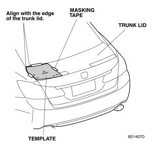
12. Using a felt-tip pen, mark the trunk lid through the two holes in the template. Remove the template.
