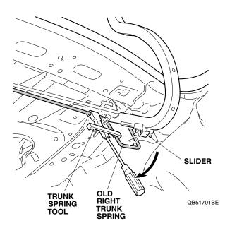
• Remove the old right trunk spring from the hinge bracket.
