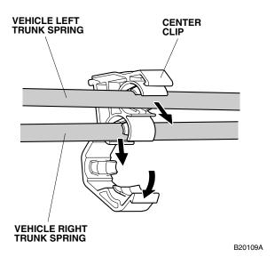
42. With an assistant holding the trunk lid open, remove the old right trunk spring from the slider using the trunk spring tool. Wear gloves to protect your hands, and push the trunk spring tool slowly and carefully.
