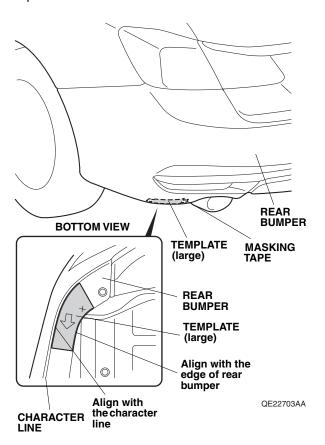
4. Place the left template on the rear bumper in the area shown, and attach it with masking tape.
