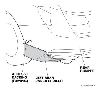
Using your hand, firmly press the left rear under spoiler against the rear bumper for 30 seconds. 20. Using a rubber roller, apply firm pressure while rolling to set the adhesive, especially at the ends.
