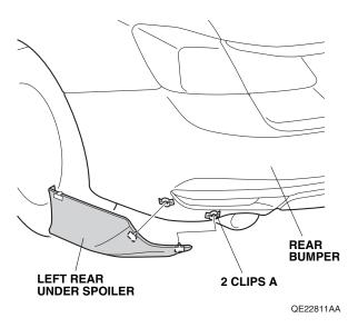
17. Loosely secure the left rear under spoiler to the rear bumper with two self-tapping screws.
