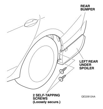
18. While applying light pressure against the left rear under spoiler, carefully remove the adhesive backing.
