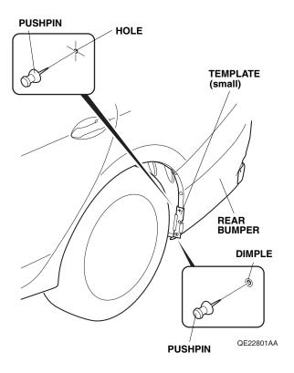
6. Using a pushpin, pierce the rear bumper through the hole in the template. Remove the template.
