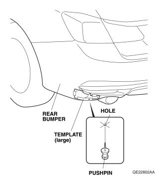
7. Using a pushpin, pierce the rear bumper through the two holes in the left template. Remove the left template.
