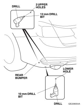
10. Enlarge the lower hole to 10 mm using a 10 mm drill bit. Remove any burrs.
