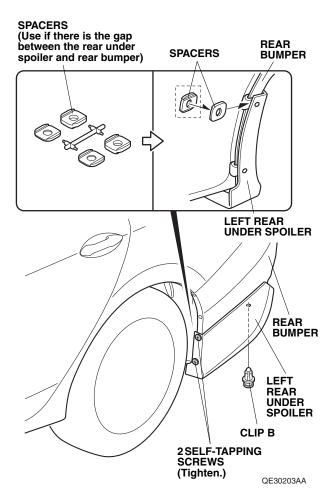
22. Turn the template over and repeat steps 2 through 21 to install the right rear under spoiler.
