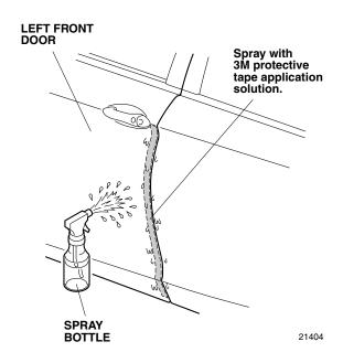
Open the left front door. Peel back about 50 mm (2.0 in.) of adhesive backing from the left front door edge film. Align the V-notch on the left front door edge film with the character line on the left front door.
