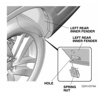
10. Loosely install the left rear splash guard to the rear bumper and left rear inner fender with two 5 x 20 mm self-tapping screws and the two self-tapping screws removed in step 7.
