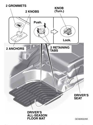
2. Place the grommets in the driver's all-season floor mat over the anchors. Push the grommets into the anchors to secure the retaining tabs, then turn the knobs 90° to secure the all-season floor mat.
