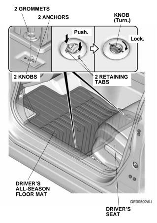
2. Place the grommets in the driver's all-season floor mat over the anchors. Push the grommets into the anchors to secure the retaining tabs, then turn the knobs 90° to secure the all-season floor mat.
