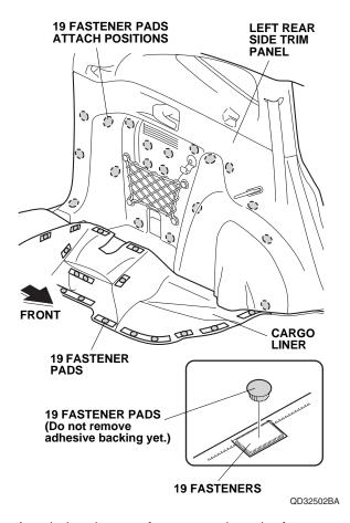
Attach the nineteen fastener pads to the fasteners on the left side of the cargo liner. 6. Using an alcohol swab, thoroughly clean the areas where the fastener pads will attach.
