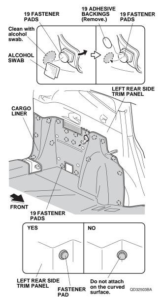
7. Remove the adhesive backing from each fastener pads, and attach them to the left rear side trim panel. Using your fingers, firmly press each fastener pads against the left rear side trim panel over the left cargo liner.
