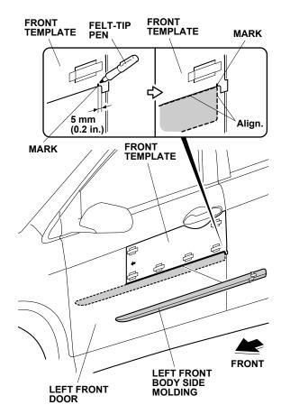
7. Align the left front body side molding with the front template and the mark you made on the front template, and attach it to the left front door as shown.
