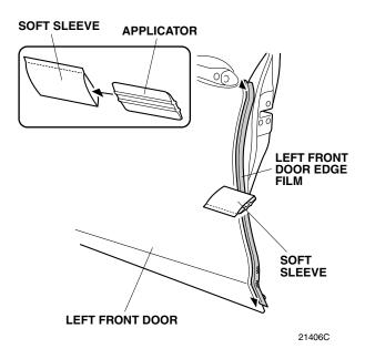
9. Slowly remove the protective film from the left front door edge film.
