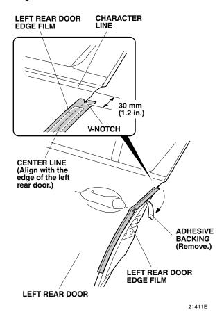
14. Align the center line on the left rear door edge film to the edge of the left rear door. While applying light pressure, carefully remove the adhesive backing.
