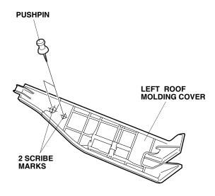
3. While wearing eye protection, drill two holes in the left roof molding cover with a 3 mm drill bit at the pierced marks made in step 2.
