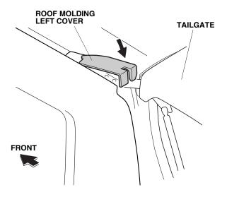
12. Reinstall the roof moldings back into the left roof channel using the two new roof molding clips installed in step 10.
