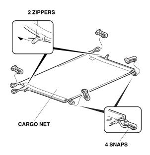
6. Attach four snaps onto the cargo net as shown.
