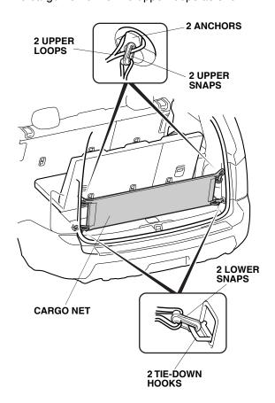
8. Attach the two lower snaps on the cargo net to the two tie-down hooks.
