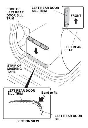
9. Using the palm of your hand, press the left rear door sill trim firmly against the door sill, and remove the adhesive backings. Apply firm pressure, especially at the ends.
