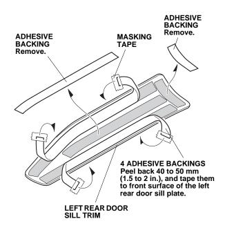
8. Starting at the curved area, bend the left rear door sill trim against the left rear door sill. Align the edge of the left rear door sill trim with the masking tape, and install the left rear door sill trim.
