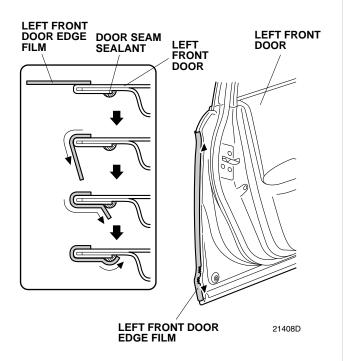
11. Using a shop towel, wipe the excess 3M protective tape application solution from the left front door edge film. Allow the left front door edge film to dry thoroughly.
