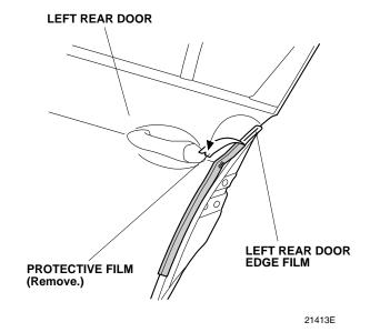
17. Starting from the center and working outward, use your finger to fold the left rear door edge film inside the left rear door. Move the your finger in one direction only. Do not damage the door seam sealant.
