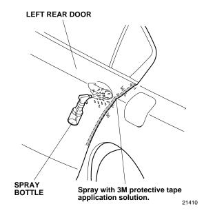
Open the left rear door. Peel back about 50 mm (2.0 in.) of adhesive backing from the left rear door edge film. Align the V-notch on the left rear door edge film with the left rear door as shown.
