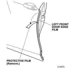
10. Starting from the center and working outward, use your finger to fold the left front door edge film inside the left front door. Move the your finger in one direction only. Do not damage the door seam sealant.
