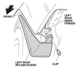
4. Install the left rear splash guard with two self-tapping screws in the order as shown. Make sure that there is no gap between the rear bumper and the splash guard before tightening the screws.
