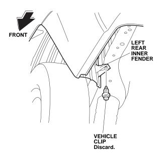
3. While holding the left rear splash guard against the vehicle, secure the splash guard with a new clip.
