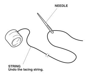
Starting at the back of the left spoke, lace the string through the holes of the steering wheel cover from the inside. Leave approximately 100 mm (3.93 in.) of string at the end. This will be used to tie the string when finished.
