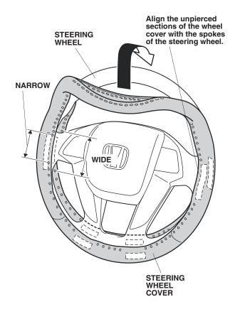
3. Pull back the edge of the steering wheel cover. Peel back the adhesive backings shown, and temporarily attach them to the front of the steering wheel cover with masking tape.
