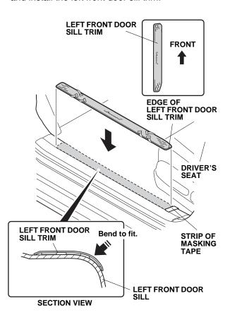
6. Using the palm of your hand, press the left front door sill trim firmly against the door sill, and remove the adhesive backing in the order shown. Apply firm pressure, especially at the ends.
