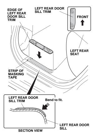
Using the palm of your hand, press the left rear door sill trim firmly against the door sill, and remove the adhesive backings. Apply firm pressure, especially at the ends.
