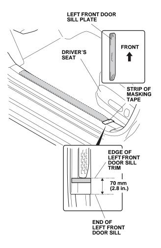
2. Open the left rear door. Place the door sill trim on the door sill at the measurement shown, and mark the door sill using a strip of masking tape at the edge of the door sill trim.
