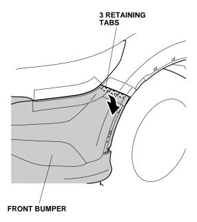
• On each side, release the four retaining tabs.
