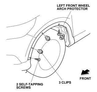
6. Remove the left front wheel arch protector (eight clips and three retaining tabs).
