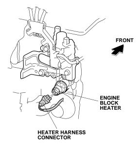
40. Align the mark at point A with the vehicle clip, and secure the heater harness to the vehicle harness with white wire tie.
