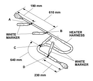
Plug the heater harness connector to the engine block heater. Make sure that the heater harness connector is properly installed.
