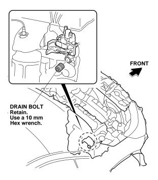
37. Install the new aluminum washer and the engine block heater into the bolt hole using a 24 mm socket and a torque wrench. Torque the engine block heater to 60 N·m (44 lbf·ft).
