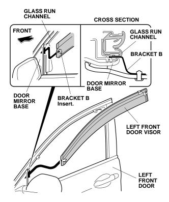
7. Align the clip holes in the left front door visor with the bracket holes, and install the clips while pushing up on each bracket A. There should be no clearance between the brackets and the door sash.
