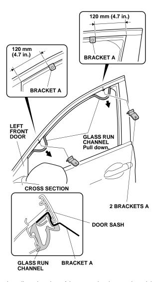
Install two brackets A between the door sash and the glass run channel at the measurements shown. Seat the glass run channel properly around the brackets. 4. Using isopropyl alcohol on a shop towel, thoroughly clean the door sash where the left front door visor will attach.
