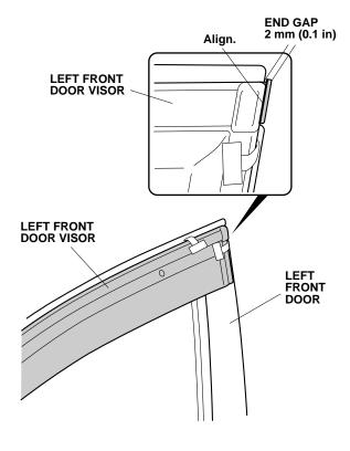
While applying light pressure against the left front door visor, carefully remove the adhesive backings in the order shown. Use your finger to push up each bracket so there is no gap between the bracket and the door sash.
