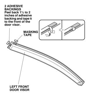
6. Position the left front door visor onto the left front door by inserting bracket B between the door mirror base and glass run channel as shown.
