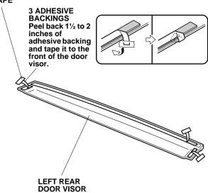
16. Align the clip holes in the left rear door visor with the bracket holes, and install the clips while pushing up on each bracket A. There should be no clearance between the brackets and the door sash. NOTE: Be sure the bracket and the door visor are aligned properly. Once the clip is installed, it cannot be reused.
