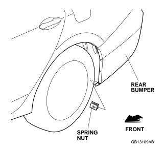
13. Install the left rear splash guard to the rear bumper with two new washer-screws and the washer-screw removed in step 7. Install them in this order
