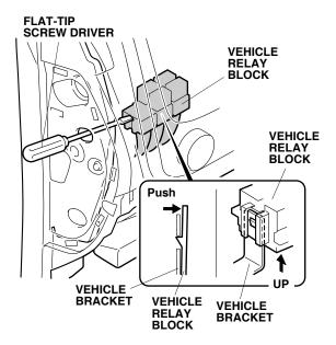
9. Plug the two relays into the vehicle relay block, and reinstall the vehicle relay block.
