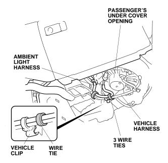
Install the ambient light into the passenger's under cover as shown.
