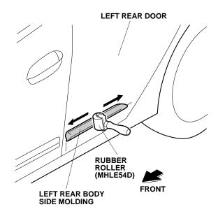
17. Turn the templates over, and repeat steps 1 thru 16 to install the body side moldings on the right side of the vehicle.
