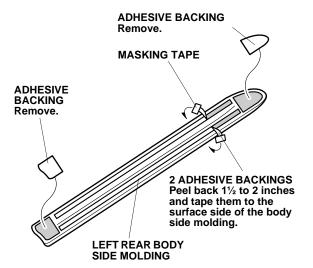
13. Align the left rear body side molding with the rear template, and attach it to the left rear door.
