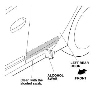
10. Align the rear template to the left rear door and attach the template to the door using masking tape.
