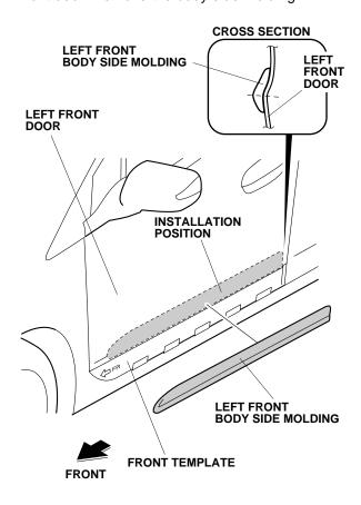
4. Peel back approximately 1½ to 2 inches of adhesive backing from each adhesive strip, and tape the ends to the front surface of the body side molding. Remove the small end pieces of adhesive backing.
