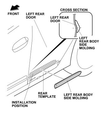
12. Peel back approximately 1½ to 2 inches of the adhesive backing from each adhesive strip, and tape the ends to the outside surface of the body side molding. Remove the small end pieces of adhesive backing.
