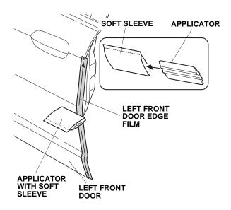
6. When you are satisfied that the door edge film is firmly attached to the door, slowly remove the outer protective film.
