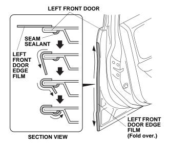
8. Using a lint-free shop towel, wipe up the liquid from the front door edge film. Allow the front door edge film to dry thoroughly.
