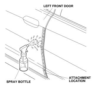
Open the left front door again. Peel back about 50 mm (2 in.) of adhesive backing from the left front door edge film. Align the V-notch in the door edge film with the end of the character line on the upper part of the front door.
