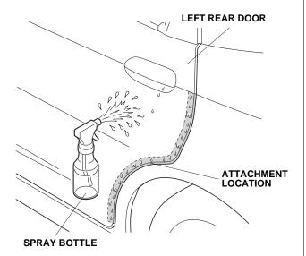
12. Open the left rear door again. Peel back about 50 mm (2 in.) of adhesive backing from the left rear door edge film. Align the V-notch in the door edge film with the end of the character line on the upper part of the left rear door.
