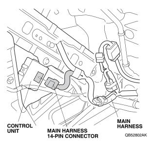
26. Using three wire ties, secure the main harness to the vehicle harness.
