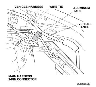
30. Using one wire tie, secure the main harness to the vehicle harness.
