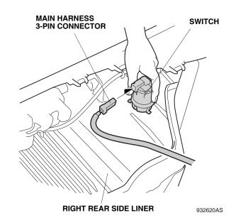
49. Reinstall the right rear quarter pillar lining, before reinstalling the right rear side liner. Be careful not to bump the switch during installation.
