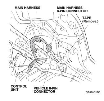
25. Plug the main harness 14-pin connector into the control unit as shown.
