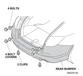
• On each side, remove the four self-tapping screws at the fenderwell.
