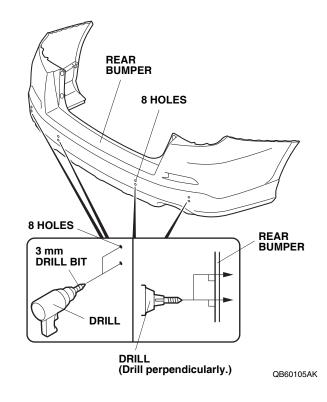
52. While wearing eye protection and drilling from outside of the rear bumper, enlarge the two lower 3 mm outer holes to 24 mm using a 24 mm hole saw. NOTE: Make sure to drill perpendicularly to the rear bumper. Remove any burrs.
