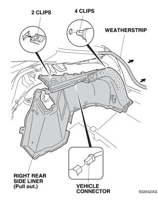
19. Pull away the weatherstrip and door seal from around the right rear quarter pillar lining. Remove the right rear quarter pillar lining (one self-tapping screw and seven clips). Be careful not to crease the headliner.
