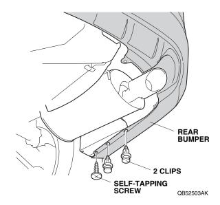
With the help of an assistant, remove the rear bumper. Place the rear bumper on a blanket to prevent damage.
