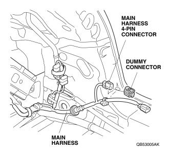
38. Route the main harness through the hole in the order shown. Set the main harness grommet into the vehicle panel.
