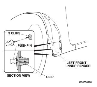
2. Using a pushpin, pierce the centers of the three clips shown on the left front inner fender.
