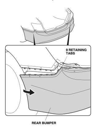
With the help of an assistant, remove the rear bumper (four retaining tabs). Set the rear bumper on a blanket to prevent damage.
