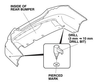
4. Use a deburring tool to remove any burrs from the holes.
