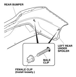
11. Align the left rear under spoiler to the rear bumper as shown. Make sure there are no gaps.
