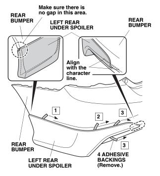
12. Remove the four adhesive backings in the order shown. Press the left rear under spoiler firmly against the rear bumper with the palms of your hands to set the adhesive.
