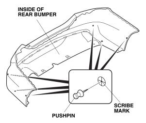
3. While wearing eye protection, drill the two lower pierced marks with a 3 mm drill bit, then enlarge the holes with a 10 mm drill bit.
