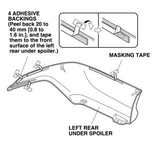
9. Install the left rear under spoiler with one bumper clip.
