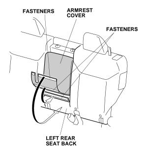
9. Secure the fastener to the bottom of the left rear seat back. Return the left rear seat cushion to its original position. Reinstall the center headrest.
