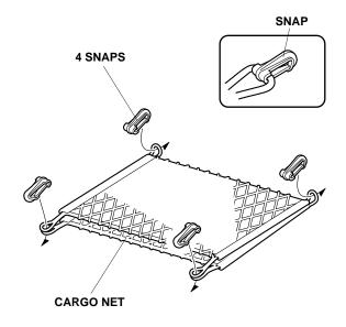
2. Open the tailgate, and secure four snaps to the hooks in the cargo area.
