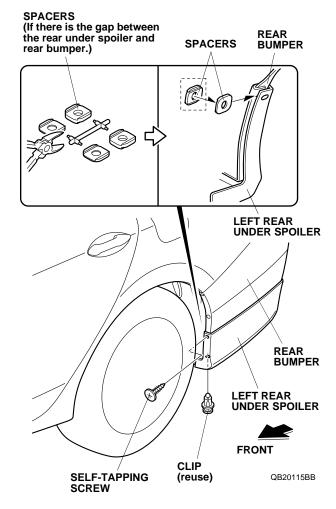
21. Repeat steps 1 through 20 to install the right rear under spoiler on the right side of the vehicle.
