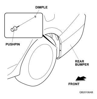
9. Thread a self-tapping screw into the pierced mark to make a hole in the rear bumper. Remove the self-tapping screw.
