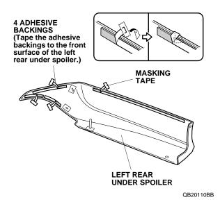
12. Install three seals onto the clip on the left rear under spoiler.
