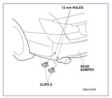
8. Using a pushpin, pierce the rear bumper at the dimple on the rear fenderwell.
