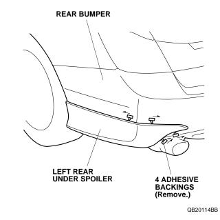
18. Using your hand, firmly press the left rear under spoiler against the rear bumper for 30 seconds.
