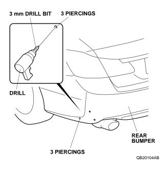
5. Enlarge the two upper holes to 12 mm using a 12 mm drill bit. Remove any burrs.
