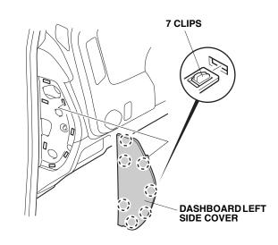
8. Insert a flat-tip screwdriver wrapped with a shop towel into the grooves in the instrument panel and release the two clips. Pull the instrument panel out toward you to release the 18 clips. Unplug the vehicle conectors, and remove the instrument panel.
