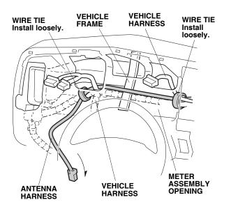
23. Route the antenna harness along the vehicle harness and secure it to the vehicle harness with four loosely-installed wire ties.
