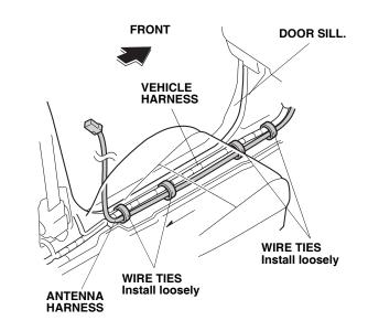
25. Route the antenna harness and the bus cable under the floor carpet. Pull them out of the cutout in the floor carpet.
