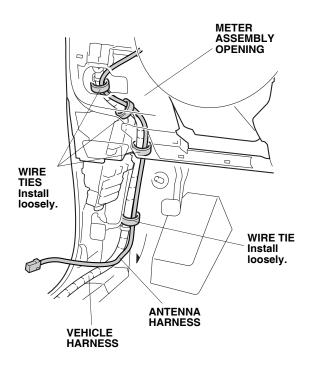
24. Route the antenna harness as shown and secure it to the vehicle harness with four loosely-installed wire ties.
