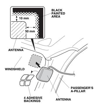
16. Route the antenna harness down the passenger's A-pillar along the vehicle harness. Secure the antenna harness to the vehicle harness with three wire ties in the areas shown.
