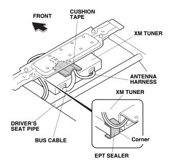
33. Attach the EPT sealer to the corner of the XM tuner as shown.
