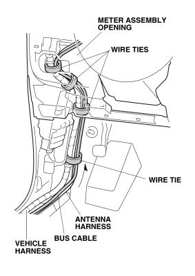
36. Route the bus cable as shown. Secure the bus cable and antenna harness to the vehicle harness by tightening the two wire ties loosely-installed in step 22.
