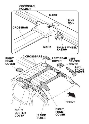
12. Loosen four thumb wheel screws on the crossbar holders. Align the marks on the crossbar holders with the marks on the side rails. Securely tighten the thumb wheel screws.
