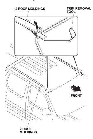
Slide and remove the two roof moldings from the vehicle.
