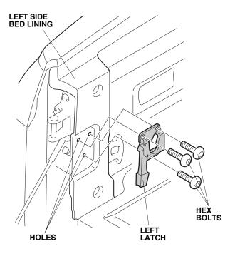
2. Install the left latch to the left side bed lining with three hex bolts.
