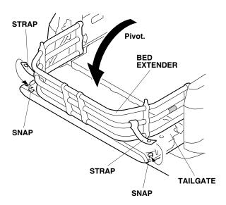
21. Secure two straps on the bed extender to two snaps on the tailgate.
