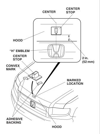
Remove the adhesive backing from the center stop, and attach it to the hood at the marked location with the convex mark facing down. 3. Open the hood. Locate the outer four clips that attach the rubber molding. Remove the four clips from the rubber molding.
