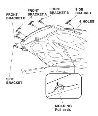
7. Attach a piece of masking tape to the hood under each bracket.
