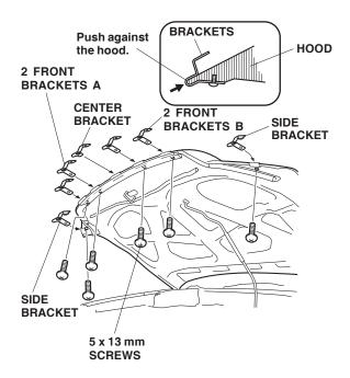
12. Install the center bracket over the hood around the protective tape.
