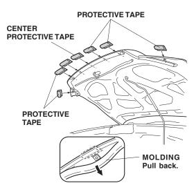
10. Attach the remaining protective tape around the center of the front edge of the hood. Remove the masking tape.
