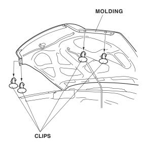
4. Pull back the rubber molding and locate the six square holes in the hood. Push one plastic grommet into each square hole.
