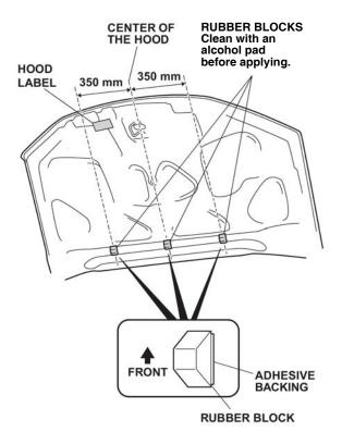
Remove the adhesive backings from three rubber blocks and hood label and attach them to the hood at the measurements shown. 7. Close the hood. Using an alcohol pad, thoroughly clean the hood where the bracket C will attach.
