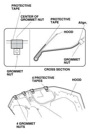
3. Remove the adhesive backings from each protective tapes and attach the four protective tapes around the front of the hood as shown.
