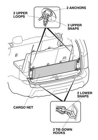
8. Attach the two lower snaps on the cargo net to the two tie-down hooks.
