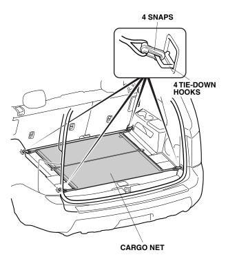
4. Attach four snaps on the cargo net to the four tie-down hooks in the cargo area.
