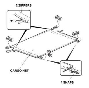
6. Attach four snaps onto the cargo net as shown.
