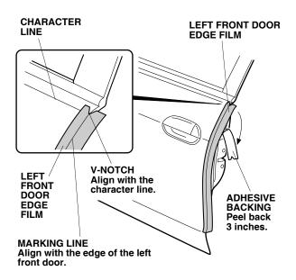
7. When the alignment is correct, apply light pressure to the door edge film while you carefully remove the adhesive backing. Don't worry about wrapping the door edge film around the door at this time.
