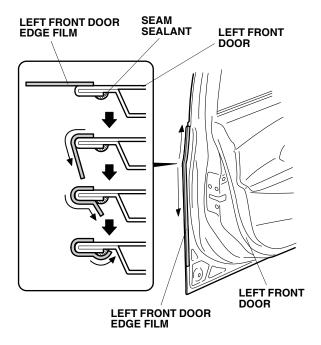
11. Using a shop towel, wipe the 3M protective tape application solution from the left front door edge film. Allow the left front door edge film to dry thoroughly.
