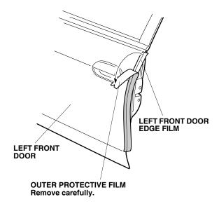
Starting from the center and working outward, fold the left front door edge film around the left front door edge. Be careful not to damage the door seal during this procedure.
