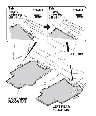
4. Install the right and left rear floor mats. Insert the tab from each floor mat under the sill trim.
