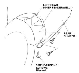
7. Secure the left rear splash guard with two 5 x 25 mm self-tapping screws and one 5 x 20 mm self-tapping screw, in the order shown.
