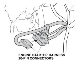
61. Attach the engine starter harness 20-pin connector to the vehicle panel as shown.
