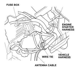
70. Bundle up the excess antenna cable as shown.
