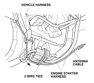
68. Plug the antenna cable terminal into the control unit as shown.
