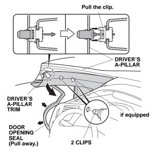
11. Pull out the driver's A-pillar trim to release the clips.
