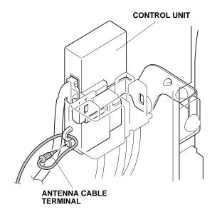
69. Using one wire tie, secure the antenna cable and engine starter harness to the vehicle harness.
