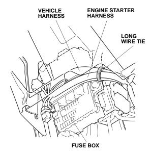
84. Cut one urethane tape, then wrap the urethane tape around the engine starter harness 5-pin connector as shown.
