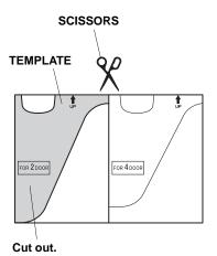
29. Attach the template to the windshield black ceramic as shown.
