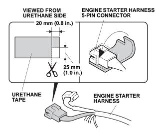
85. Unplug the vehicle 5-pin connector from the fuse box. Plug the engine starter harness 5-pin connector into the fuse box 5-pin connector. Plug the vehicle 5-pin connector into the engine starter harness 5-pin connector.
