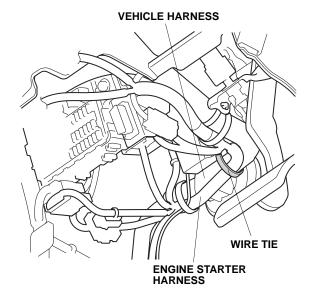
73. Route the engine starter harness along the vehicle harness as shown.
