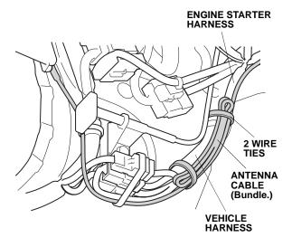
71. Using two wire ties, secure the antenna cable and engine starter harness to the vehicle harness.
