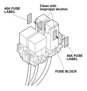
45. Attach the two 40A fuse labels to the engine starter harness fuse block.
