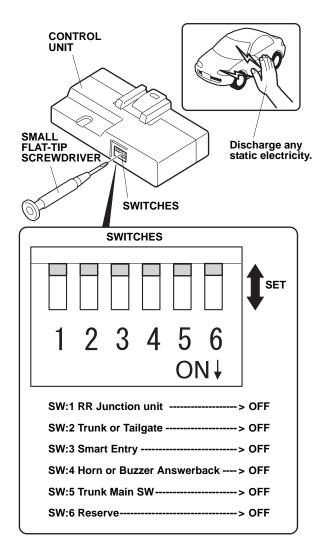
3. Using a small flat-tip screwdriver, change the dip switches on the control unit to the settings shown above.
