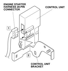
49. Install the control unit bracket to the control unit.
