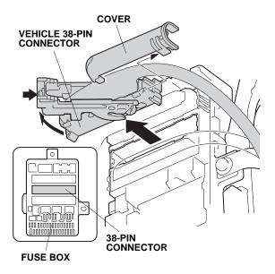
77. Remove the lever from the vehicle 38-pin connector as shown.
