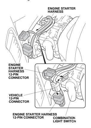
97. Using two wire ties, secure the engine starter harness to the vehicle harness. Do not secure it to the SRS harness.
