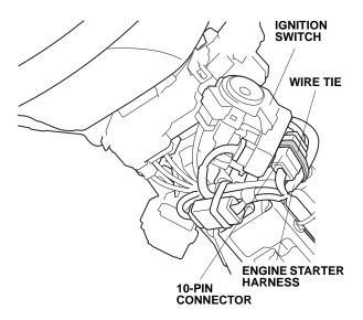
96. Route the engine starter harness as shown. Unplug the vehicle 12-pin connector from the combination light switch, and plug it into the engine starter harness 12-pin connector. Plug the remaining engine starter harness 12-pin connector into the combination light switch.
