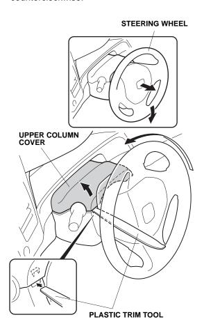
22. Using a plastic trim tool, release the lock as shown.
