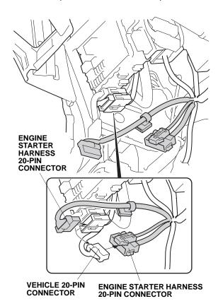
60. Plug the engine starter harness 20-pin connector to the engine starter harness 20-pin connector as shown.
