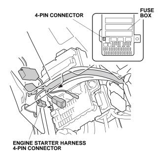
74. Plug the engine starter harness 4-pin connector into the fuse box.
