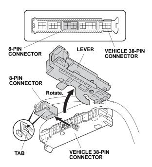
78. Remove the 8-pin connector from the vehicle 38-pin connector (two tabs).
