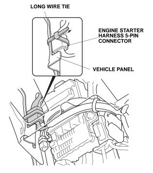
87. Route the engine starter harness as shown. Using one wire tie, secure the engine starter harness at the white tape to the hole in the instrument panel.
