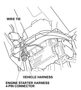
76. Unplug the vehicle 38-pin connector from the fuse box as shown. Remove the cover.
