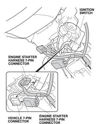
93. Using one wire tie, secure the 7-pin connector and engine starter harness to the vehicle harness.
