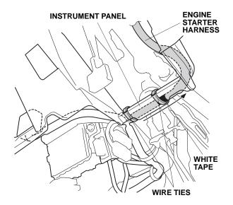
88. Using one wire tie, secure the engine starter harness to the hole in the instrument panel.
