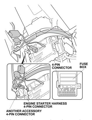
75. Using one wire tie, secure the engine starter harness 4-pin connector to the vehicle harness.
