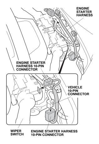
95. Using one wire tie, secure the 10-pin connector and the engine starter harness to the vehicle harness.
