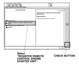
9. The following message will display: **Obtain PCM** code (IMMOBILIZER PCM CODE) from iN. This vehicle's VIN will be required to obtain the password (USA). Click on the check button.
