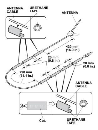
32. Cut two urethane tapes in half. Wrap the four halves of urethane tape around the antenna cable at the measurements shown.
