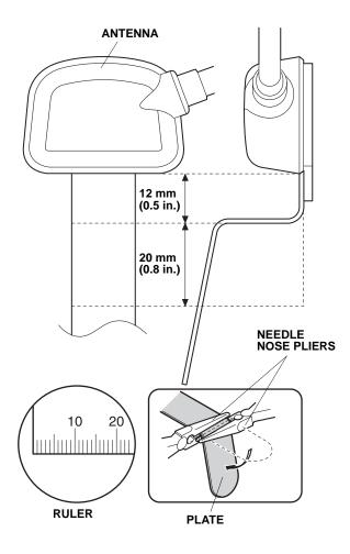
31. Starting at the antenna end of the cable, wrap three urethane tapes around the antenna cable at the measurements shown.
