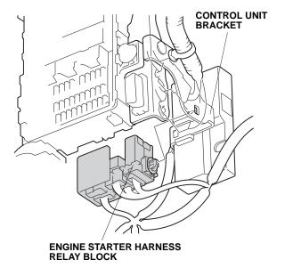
58. Align the white tape on the engine starter harness with the clip on the vehicle harness, and secure the engine starter harness to the vehicle harness with one wire tie.
