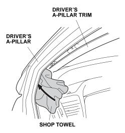
13. Remove the driver's A-pillar trim from the upper clip (unplug the vehicle connector, if equipped). Carefully remove the shop towel and any clips that fell from the driver's A-pillar trim.
