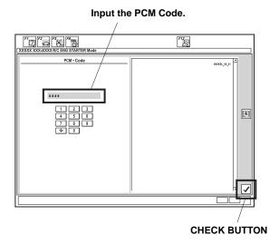
11. The following message will display: The registration of the Remote Control Engine Starter Unit has been completed. Click on the check button.
