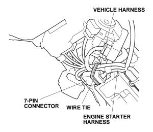
94. Route the engine starter harness as shown. Unplug the vehicle 10-pin connector from the wiper switch, and plug it into the engine starter harness 10-pin connector. Plug the remaining engine starter harness 10-pin connector into the wiper switch.
