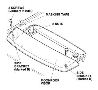
13. Position the moonroof visor with equal spacing on all sides. Check that the rubber molding is not twisted or rolled under the moonroof visor.
