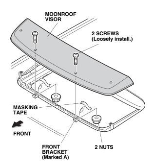
12. Loosely install the moonroof visor to the side brackets (marked B) with two screws and two nuts. Remove the masking tape.
