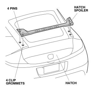
19. While applying light pressure to the hatch spoiler, carefully remove each adhesive backing in the order shown.
