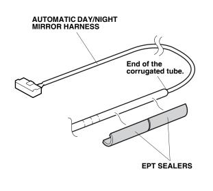
23. Attach a piece of wire to the automatic day/night mirror harness connector, then wrap electrical tape around the wire and the automatic day/night mirror harness. Route the harness to the left A-pillar trim opening.
