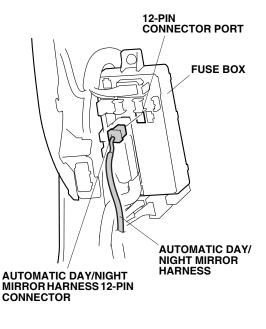
If another accessory connector is plugged into the 12-pin connector, remove the dummy connector from the other 12-pin connector harness and connect the automatic day/night mirror harness 12-pin connector into the other accessory harness.
