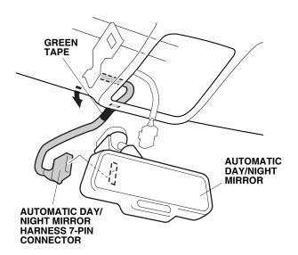
27. Align the green tape on the automatic day/night mirror harness with the edge of the roof liner. Route the automatic day/night mirror harness through the grooves in the harness cover. Attach the harness cover to the mirror stay.
