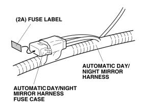
34. Plug the automatic day/night mirror harness 12-pin connector into the fuse box 12-pin connector port.
