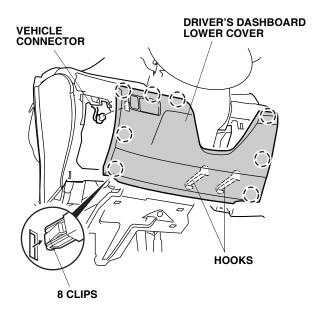
15. V6 only: Remove the driver's dashboard under cover (three clips and one pin).
