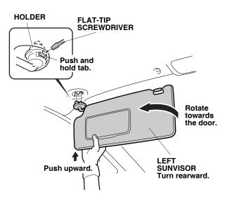
9. While holding the retaining tab, push up on the left sunvisor and rotate it towards the door to remove the sunvisor. Disconnect the vanity mirror light connector.
