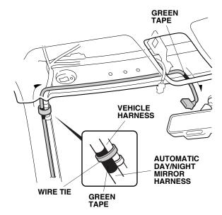
25. Route the automatic day/night mirror harness as shown. Secure the automatic day/night mirror harness to the vehicle harness at the green tape with one wire tie.
