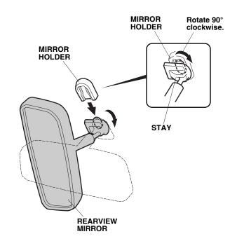
21. Replace the spring. Slide the automatic day/night mirror stay onto the mirror holder, then turn the mirror stay counterclockwise as shown.
