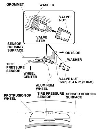
VIEWED FROM THE INSIDE OF THE ALUMINUM WHEEL 7. While holding the tire pressure sensor to keep it from rotating, torque the valve nut to 4 N·m (0.4 kgf·m, 3 lbf-ft). You may hear a snap or pop as you torque the nut; this is normal.
