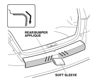
14. Remove the protective film from the top rear bumper applique. Slowly pull the protective film back as you go; do not pull it upward.
