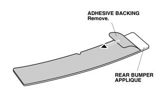
6. Spray the rear bumper applique with protective tape application solution.
