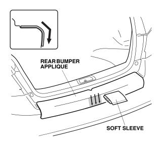
13. Use the soft sleeve to apply the rear bumper applique to the rounded rear edge on the left side as shown. Start in the middle and work outward. Repeat on the right side.
