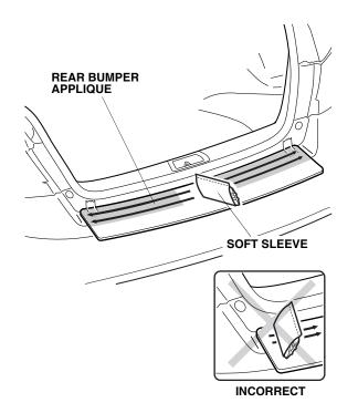
12. Once the flat surface is completely smooth with no bubbles, use the soft sleeve to apply the rear bumper applique to the rounded rear edge at the center as shown.
