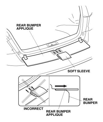
11. Starting from the center and working outward, use the soft sleeve to smooth the rear bumper applique. Repeat on the right side. Stroke in one direction only.
