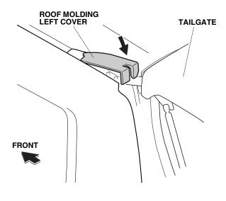
12. Reinstall the roof moldings onto the roof of the vehicle with two new roof molding clips installed in step 10.
