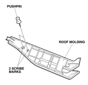
While wearing eye protection, drill two holes in the roof molding with a 3 mm drill bit at the holes made in step 2.
