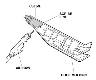
6. Remove the roof molding by carefully lifting it upward from four vehicle roof molding clips.
