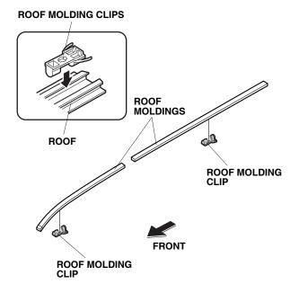
11. Reinstall the roof molding left cover.
