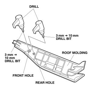
4. Enlarge the front and rear holes with a 10 mm drill bit
